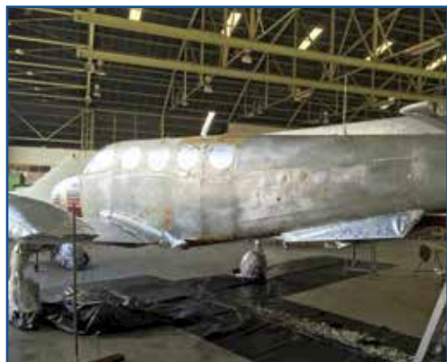
Here VVK is getting ready for paint. Note the strakes. I also installed VGs and spoilers.
