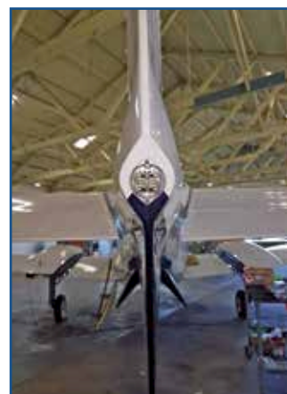
This from-behind view not only shows the strakes but one of the LED lights which replaced all the old incandescent light bulbs.
